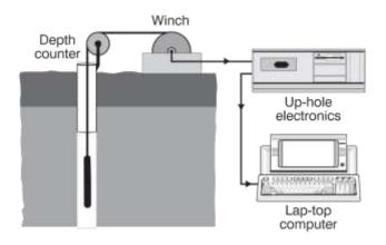
Figure 1 Schematic of a downhole sensor system (taken from Killeen, 1997)
